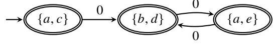
Figure 17. The observer of the DES \mathcal{A}_2 ; states marked by a double circle contain indistinguishable states of \mathcal{A}_2 .
